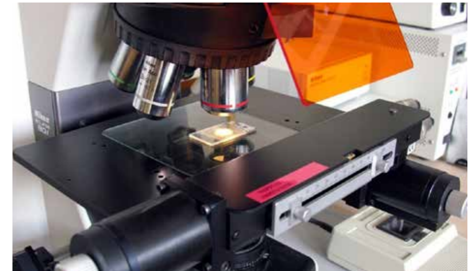
Microscopic preparation (rock thin section) in transmitted light of NIKON Eclipse 80i optical microscope
